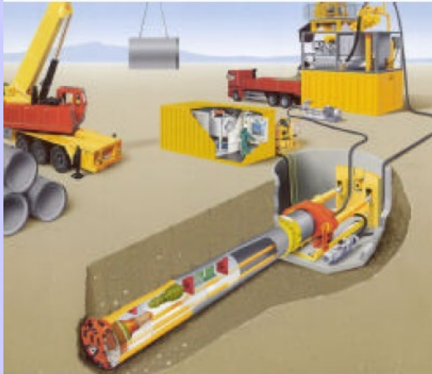
Slurry spoil removal system
