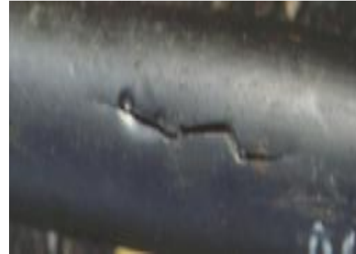
Point loading effects on 1st generation PE pipes several years after installation
