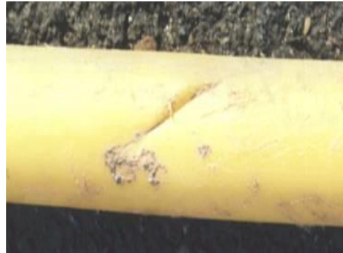
Point loading effects on 1st generation PE pipes several years after installation
